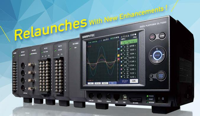
Attach up to 10 input/output modules in a mixed condition environment
